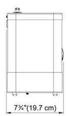
Save time and water by eliminating the wait for hot water to reach the faucet. Franke HT-400 Little Butler heating tank fits under your sink to provide precise, instant hot water between 176°F to 208°F right when you need it.
